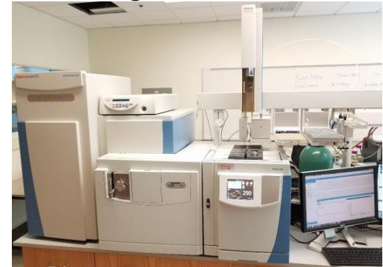
Thermo Scientific™ Q Exactive™ GC Orbitrap™ GC-MS/MS
