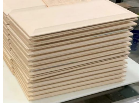
Veneer-raised panels on particleboard core (cabinet doors)
